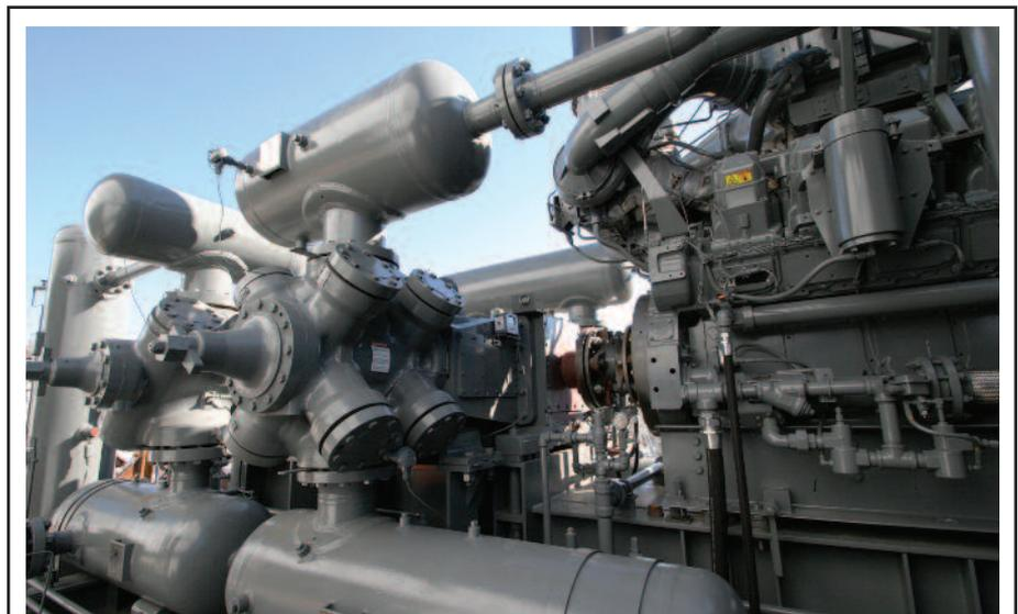
This CFH compressor from GE Oil & Gas is one of many new products designed to minimize compression-related capital and operating costs. The CFH costs less to build than a traditional compressor thanks to a low-vibration design that reduces the need for skid and pedestal material.
